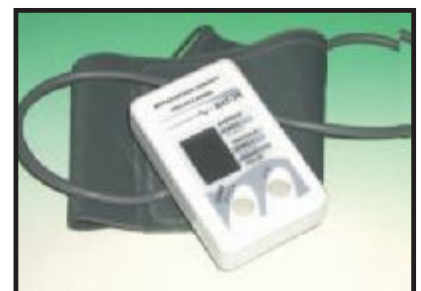
Photo 1 —Take a look at the finished product. This view of the Automatic Blood Pressure Meter shows the electronic unit box lying on the plastic air cuff.
