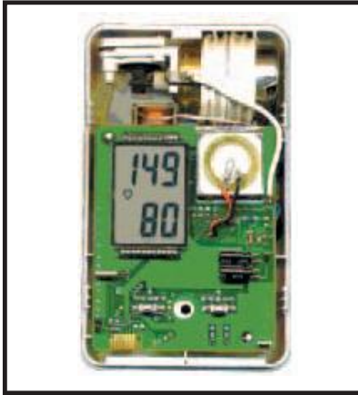
Photo 2 —We took off the blood pressure meter's front cover so you can see the placement of the electronic block's main parts. You can also see the top of the PCB.
