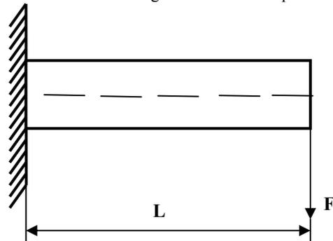
Fig. 2 Fixed beam with three degrees of freedom scheme
