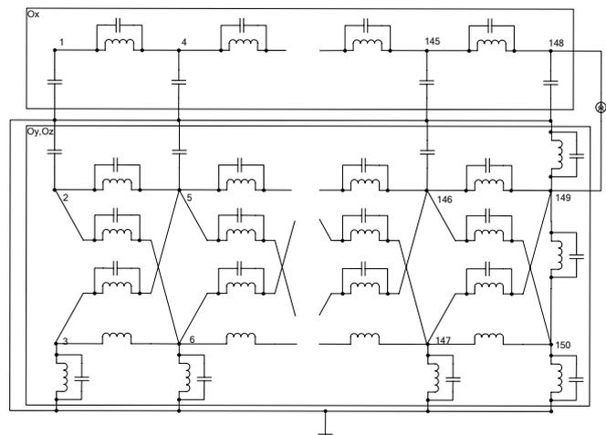
Fig. 1 Beam with three degrees of freedom equivalent circuit
