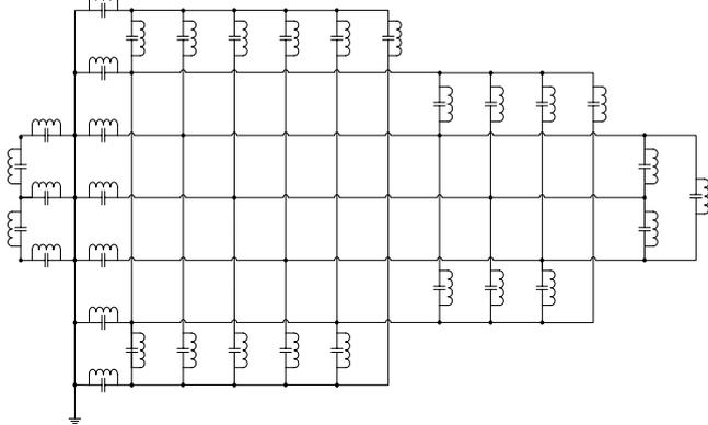
Fig. 3 Beam reduced circuit macromodel
