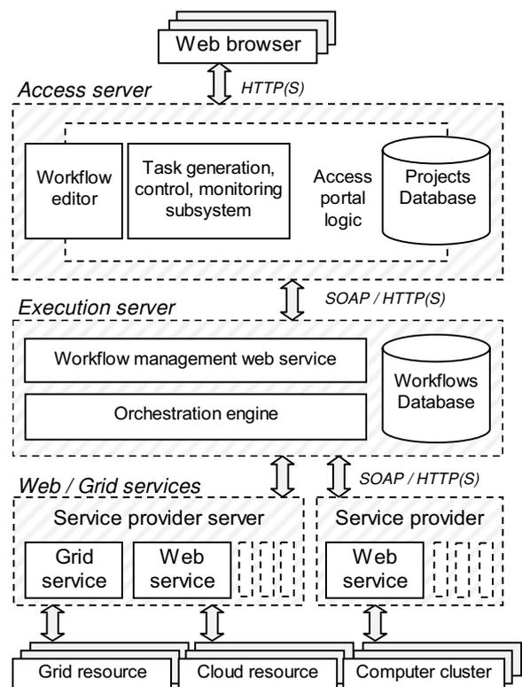
**Figure 1. General architecture layers and elements of the grid-enabled simulator**
